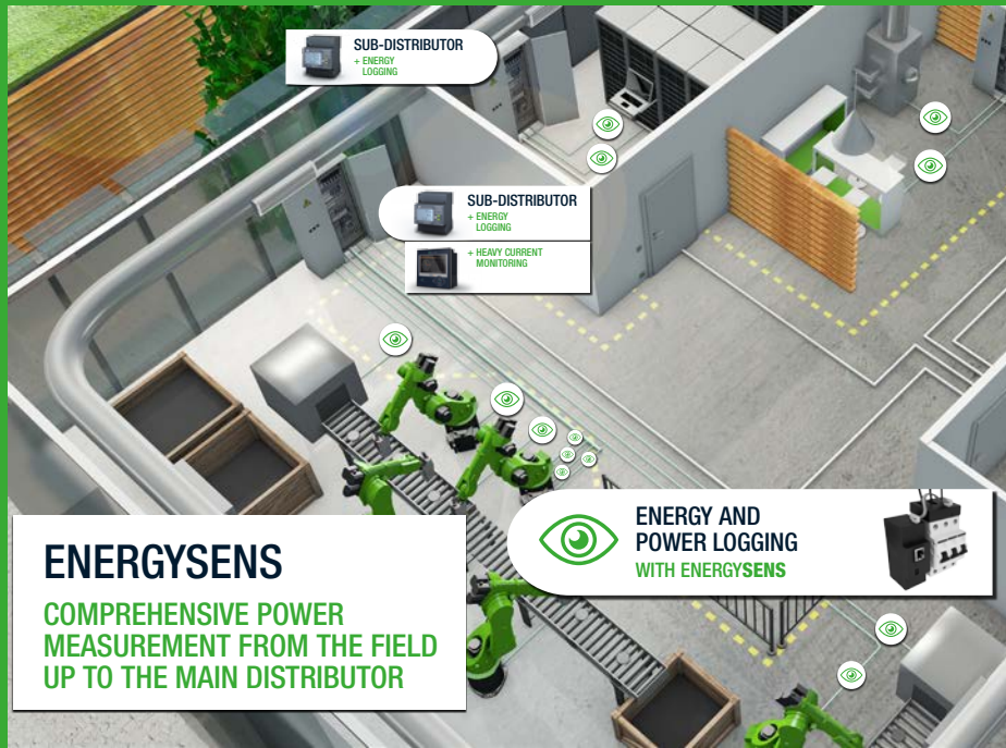
Monitoring of Phase Loads and Power Logging for Individual Production Machines
